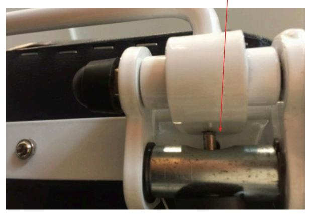
Image shows the front view of the gas strut pin. Pin should be fully extended when not activated. If it is not, head cradle will not hold.
