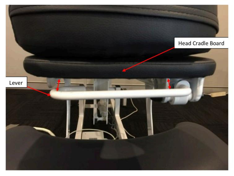
If head cradle is stiff during adjustment, lever should have slightly more clearance on the left-hand side than the right-hand side of the head cradle board. If this is not the case, hold the lever on the left-hand side and pull (bend) down.
