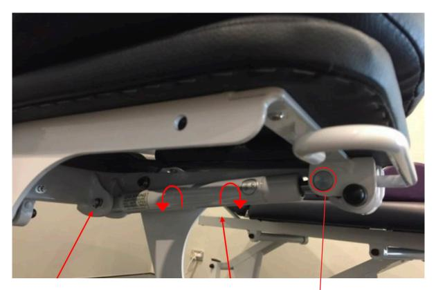
If the head cradle does not hold, remove this bolt and adjust the gas strut two turns anti-clockwise. If the head cradle does not adjust at all, adjust the gas strut two turns clockwise. Put bolt back in place.
