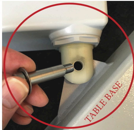
10a. Slide the actuator fork over the base mount. Push the bolt through the fork bush and the base mount bracket.
