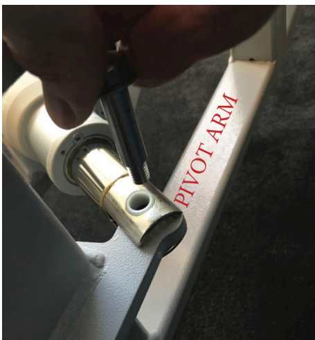
11. Slide the actuator fork over the pivot arm bracket. Push the bolt through the fork bush and the pivot arm mount bracket. You can lift or lower the pivot arm so that it is easier to push the bolt right through.
