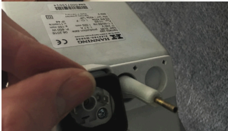
4. Remove square power connector and the black gasket (if it does not remain attached to the square connector) from the top of the actuator.
