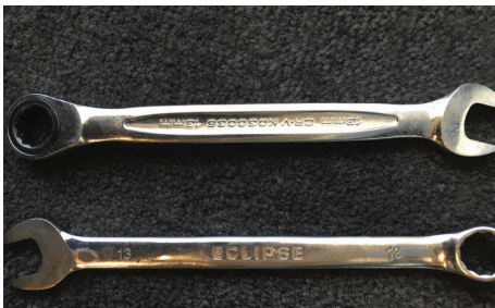
6a. Use two 13mm spanners to remove actuators fitted with shoulder bolts and nuts.
