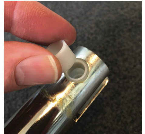
10b. Place plastic bushes into the fork at the top of the actuator (i.e. the telescopic hub fork).
