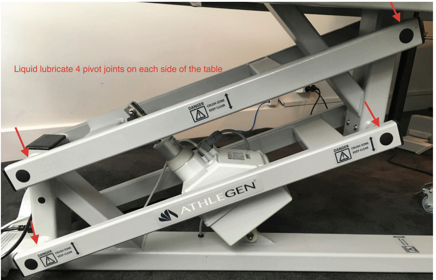
Side view: Liquid lubricate all eight pivot points
